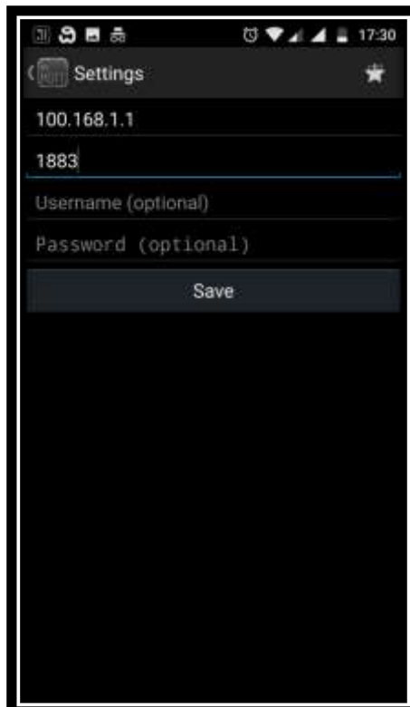
Figure 18: MQTT broker IP address and port number entered
