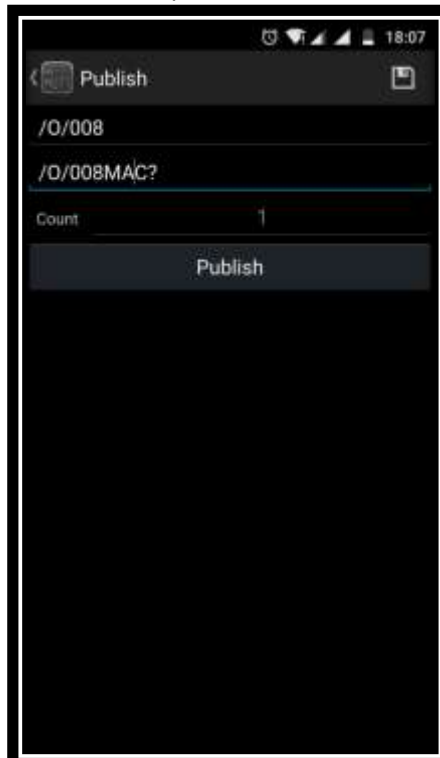
Figure 25: Entered topic and message to be Published to read the MAC address of the device
